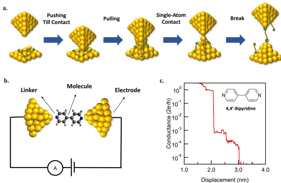
Figure 2. (a) Formation of molecular junction upon contact with a SAM (b) Scheme of STM-BJ circuit (c) Sample trace of conductance versus displacement for Au electrodes
