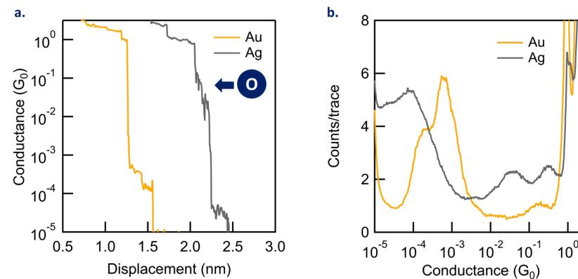
Figure 3. (a) Sample conductance traces and (b) logarithmically binned conductance 1D histograms (4000+ traces compiled without data selection) for BP measured with Au and Ag electrodes.
