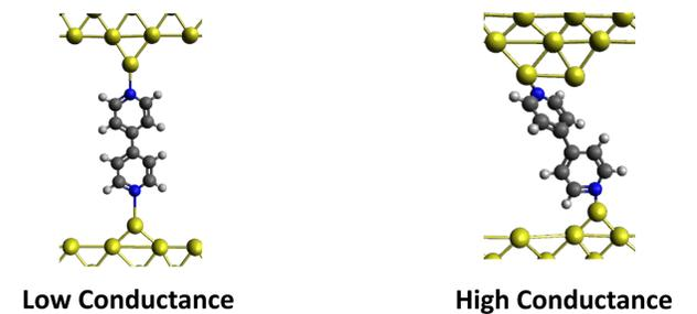
Figure 5. Potential Junction Geometries for BP measured with Au electrodes
