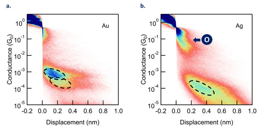
Figure 4. 2D conductance histograms measured with Au (a) and Ag (b) tips. Dashed lines are indicative of junction geometries.
