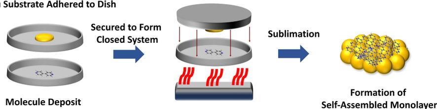
Figure 1. 4,4'-Bipyridine molecules are deposited onto Au substrates via sublimation
