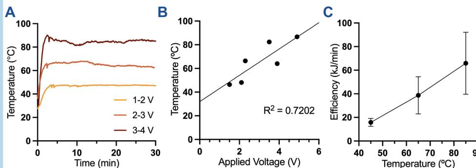
**Figure 5.** (A) Heating stability of AgNW-PLA heater. Plot shows average temperature across replicates. Each replicate (n=2) required slightly different voltage to reach target temperatures (45°C, 65°C, 85°C); voltage range shown in legend. (B) Relationship between applied voltage across copper electrodes and temperature of AgNW-PLA heater demonstrates linear pattern. (C) Efficiency (kJ/min) of AgNW-PLA heaters at different temperatures (n=4).
