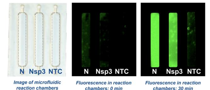
**Figure 9.** Fluorescence RT-LAMP visualizes amplification difference between SARS-CoV-2 targets (N, Nsp3) and negative control (NTC).
