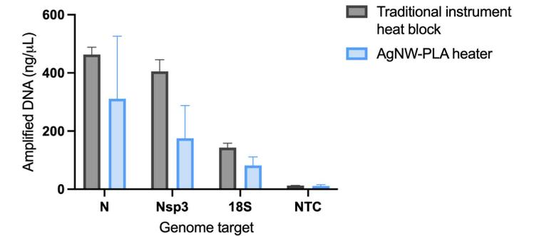
**Figure 8.** Endpoint quantification of amplified DNA from RT-LAMP assay to detect SARS-CoV-2 shows **successful amplification** of 2 SARS-CoV-2 genome targets (N, Nsp3) and positive control (human 18S rRNA), and none for negative control (NTC). Starting concentration was 10<sup>5</sup> copies/mL inactive virus spiked in human saliva (n=3).
