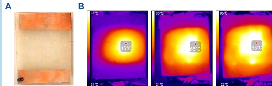
**Figure 4.** Images of AgNW-PLA heater. (A) Standard camera image demonstrates transparency of AgNW-PLA. (B) Infrared thermal images of AgNW-PLA heater across different temperatures (left to right: 45°C, 65°C, 85°C).
