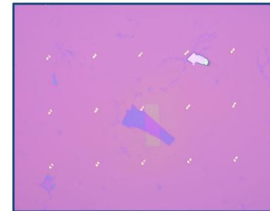
hBN on SiO<sub>2</sub> chip, "soft milled" for 5 minutes
