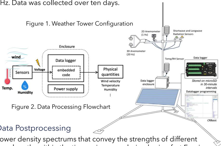
Figure 2. Data Processing Flowchart
