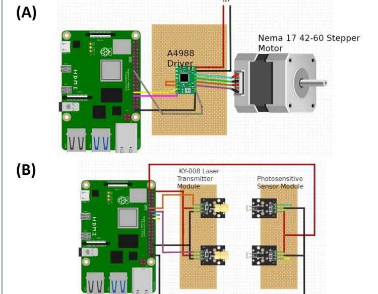
A Raspberry Pi 4 was used to control the (A) conveyor belt motor and (B) two laser sensors. When the sensor module moves into position, it blocks the laser, triggering the conveyor belt to stop moving.
