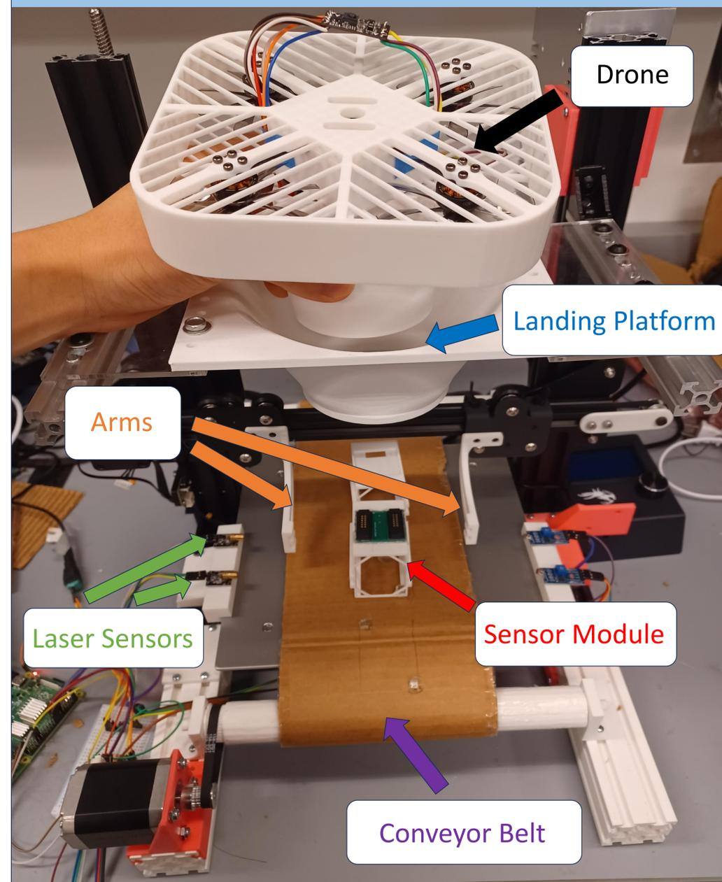
The basket-like design of the landing platform allows the drone to easily land in the correct position. The arms grab the sensor module below and attach it to the drone via a set of magnetic connectors, allowing it to fly away and execute a given task.
