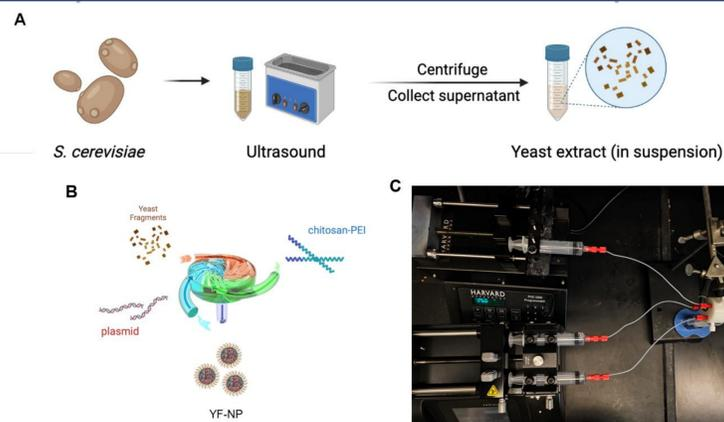
**Figure 1:** process for YNP formation. A) Yeast fragment obtained by sonicating the cells then extracting after centrifuging. B) Diagram of triple inlet FNC formation. C) Photo of experimental setup
