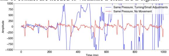
Figure 2. ECG Detection using Fabric Electrodes Attached to the Prototype Steering Wheel while Demonstrating Different Driving Techniques
