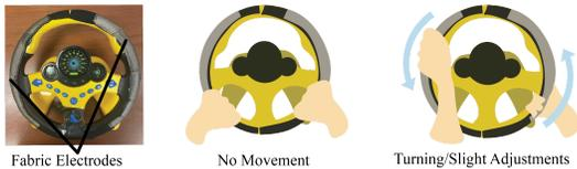
Figure 1. Steering Wheel Prototype & Different Driving Motions For Testing
