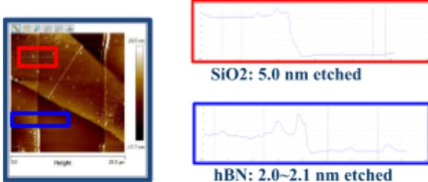
Figure 1. hBN on  $\text{SiO}_2$  chip, “soft milled” for 5 minutes
