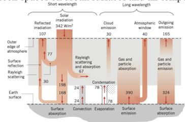
Figure 1. Breakdown of Atmospheric Energy Balance for Moderate Temperature and Cloudy Conditions
