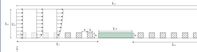
Figure 5. Diagram of the Computational Domain
