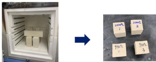
Bricks were fired at either 950°C and 1000°C in furnace for 2 hours → After firing, bricks were allowed to cool down
