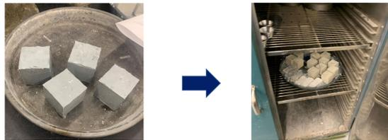
Dried in ambient conditions for 24 hours → Dried in oven at 100°C for 24 hours
