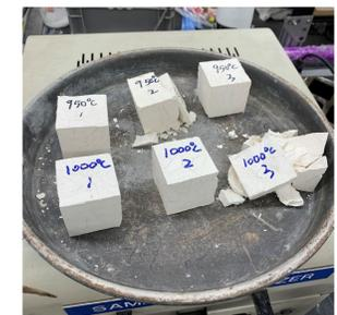
Figure 7. Bricks after firing.
