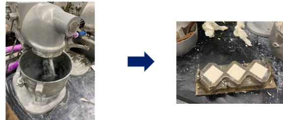
Clay-ash dry mixture mixed for 4 minutes. Water was added and mixed for 6 minutes → Mixtures pressed into three 50 x 50 x 50 mm molds and demolded
