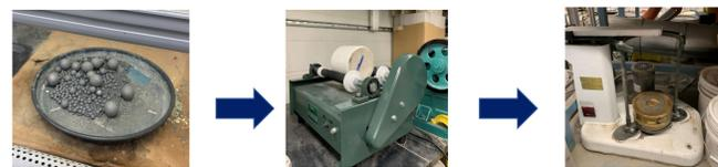
Steel balls for grinding → < 2 mm and < 9 mm WTE ash samples grinded for 2 hours in ball mill → Samples sieved through <100 um opening sieve
