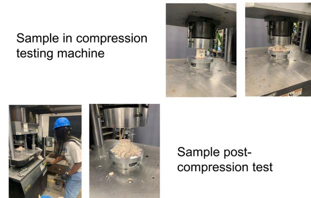
Sample in compression testing machine
