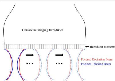
**Figure 1.** Pulse sequence of focused push and tracking pulses move electronically across lateral field to generate 2-D image<sup>6</sup>.
