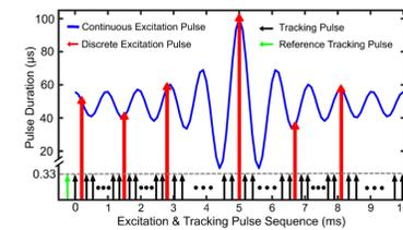
**Figure 2.** One cycle of multi-frequency ST-HMI pulse sequence with the continuous push pulse (blue) and the tracking pulses (black) in between the discrete push pulses (red)<sup>7</sup>.
