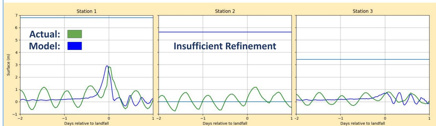
Figure 6: Comparison of simulated and actual water levels at three gauge locations.
