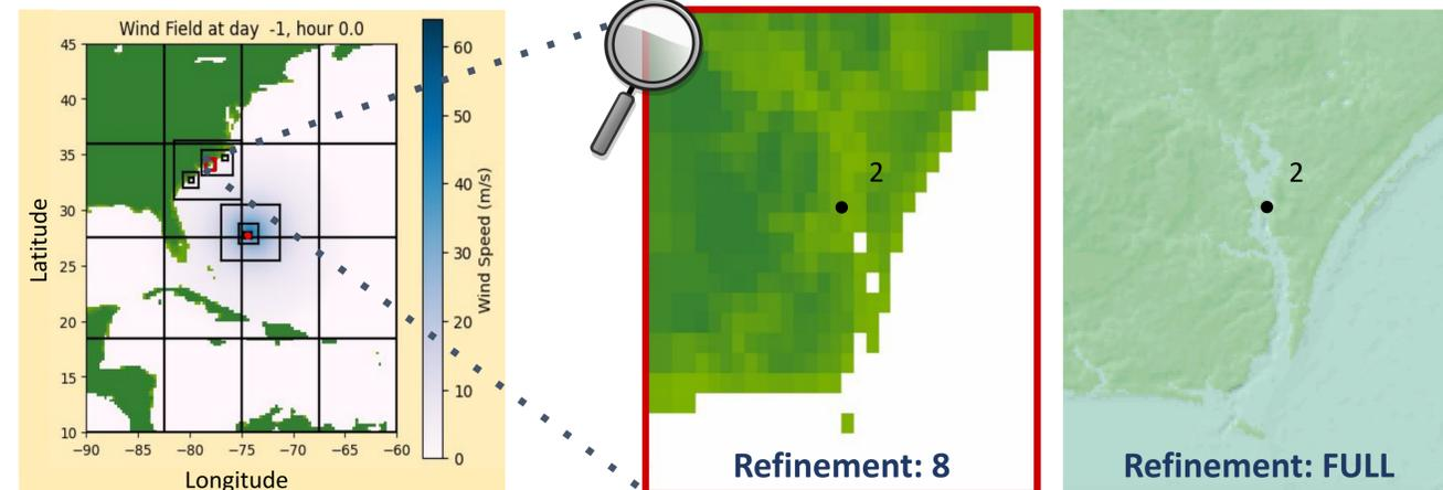
Figure 4: Boxes represent refinement areas. Smaller boxes indicate areas of forced refinement around the gauges.
