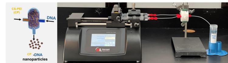
**Figure 1:** FNC apparatus used to create the NPs. The components flow from syringes into the mixing chamber, where they electrostatically complex in the turbulent flow before exiting into the test tube.
