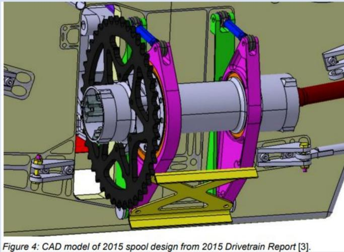
Figure 4: CAD model of 2015 spool design from 2015 Drivetrain Report [3].
