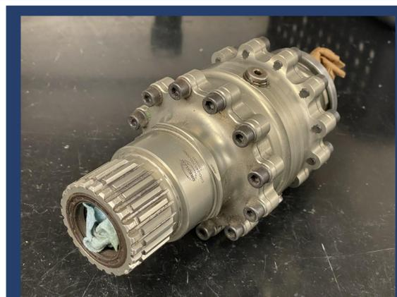
Differential Used In the Drivetrain System
