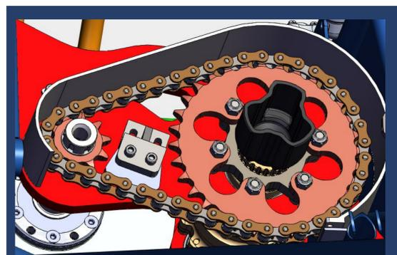
Current Design of Sprocket and Chain System with a tensioner by CUFR Team
