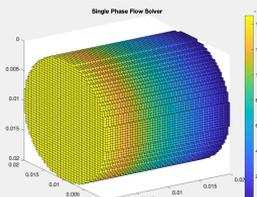
Figure 4: Pressure Gradient from Single-Phase Flow Solver
