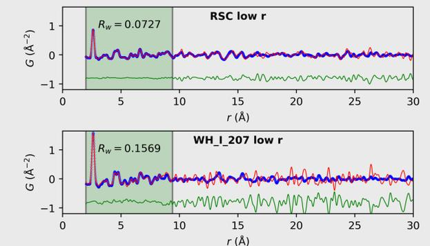
Pristine  $\text{Re}_6\text{Se}_8\text{Cl}_2$  PDF fit (top) and functionalized PDF fit (bottom)
