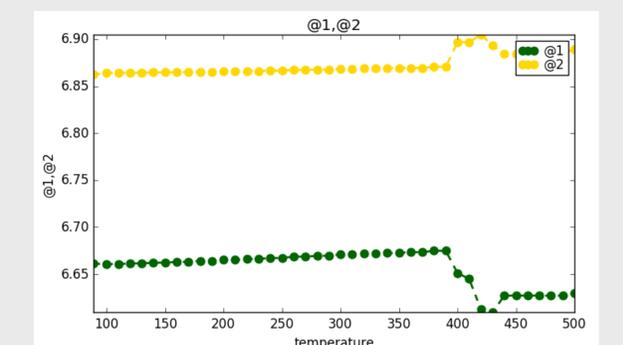
Lattice parameters of functionalized material during heating
