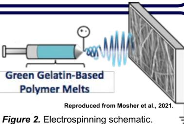
**Figure 2.** Electrospinning schematic.
