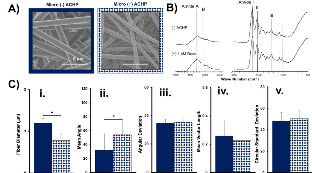
**Figure 3:** A) SEM 5000x images of (-)ACHP & (+)ACHP microfibers. B) ATR-FTIR spectrum of (-)ACHP & (+) ACHP. C) i. Fiber Diameter (n=50-60 fibers, 10-12 images). ii. Mean Vector Angle (n=10-12 images). iii. Circular Standard Deviation (n=10-12 images). iv. Angular Deviation (n=10-12 images). v. Mean Vector Length (n=10-12 images). All error bars represent standard deviation.
